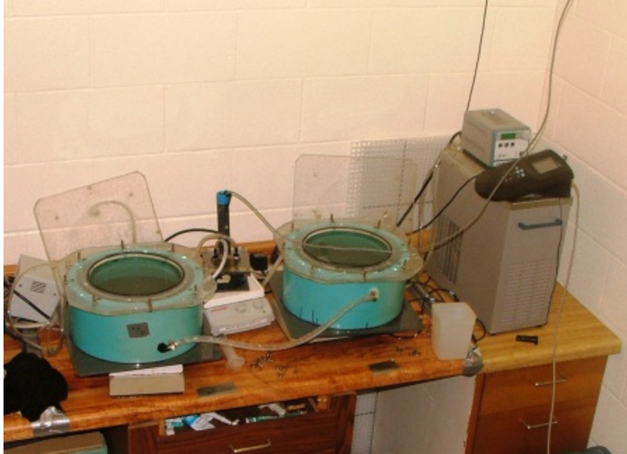
Figure 2.5. Chambers C (right) and D (left). The housing unit for the chamber D probe is between the chambers and the water chiller is the unit on the right. Note the three magnetic stir plates; one plate is under each chamber and one is under the probe housing.
