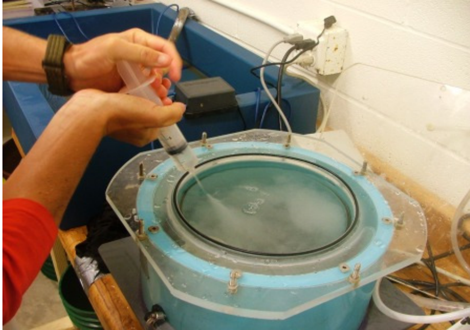
Figure 2.7. Chamber D being aerated with a 60 cc syringe.
