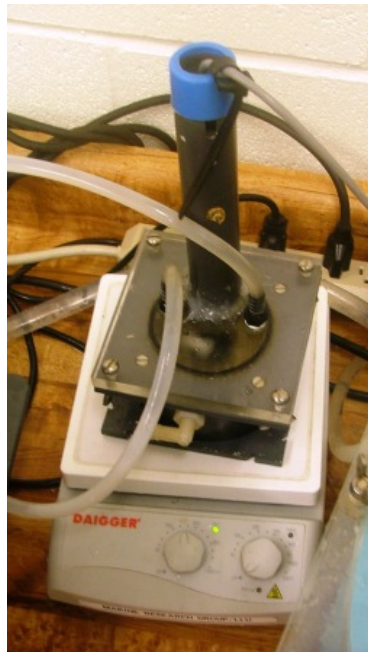
Figure 2.6. The probe housing for chamber D on top of a magnetic stir plate. Note the hoses going in and out of the housing; one goes out to the chamber and one is coming in from the peristaltic pump.
